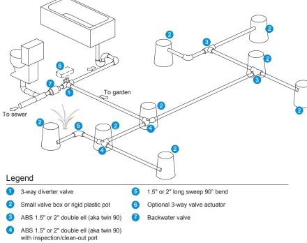
Figure 6. Branched-drain system. Source: Cleanwater Components.
