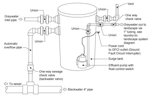
Figure 9. Drum with effluent pump.
