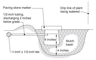
Figure 4. Mulch shield placement.
