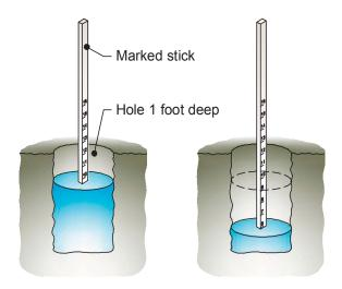
Figure 2. Drainage test.
