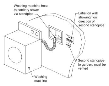
Figure 5. Second standpipe option. Source: City of Berkeley.
