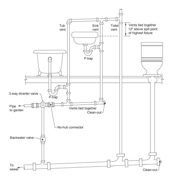
**Figure 7.** Location of the 3-way valve in a shower or sink system. Source: Art Ludwig, Oasis Design.
